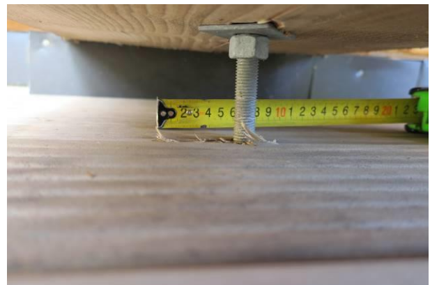
Figure 23: Sliding of the logs measured at the vertical rod.
